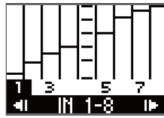
When the meters are not moving, but only the PEAK HOLD bar is displayed
