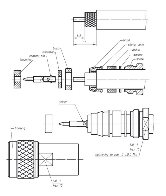
48-801 TG N CONNECTOR Male cable, solder, groups C/T Cable prep and assembly diagram
