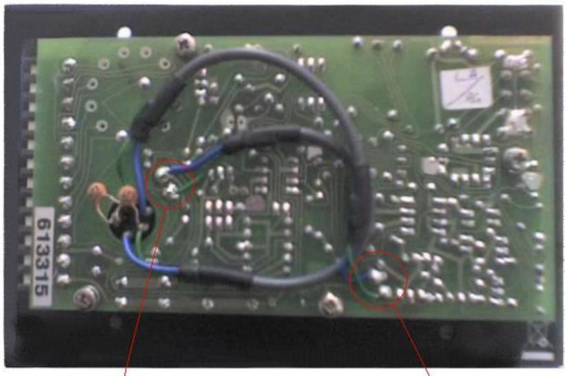
Solder pads 1.3 & 1.4 for pins for 3 & 4 from 4 pin XLR
