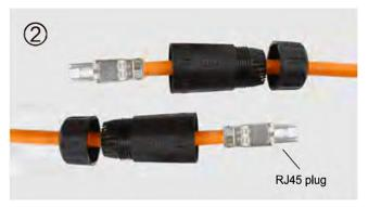
2. Pass the two cables through the end covers and the long tubes respectively.
