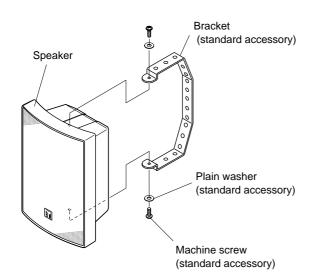
Step 2. Mount the speaker in the desired location using the mounting holes made in the bracket.
