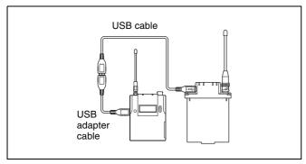
When you connect the USB cable, the encryption key is exchanged automatically, and encrypted transmission in secure key mode begins. Remove the USB cable.
