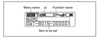
a) Indicates the power setting of the transmitter from which transmission is currently being received.
