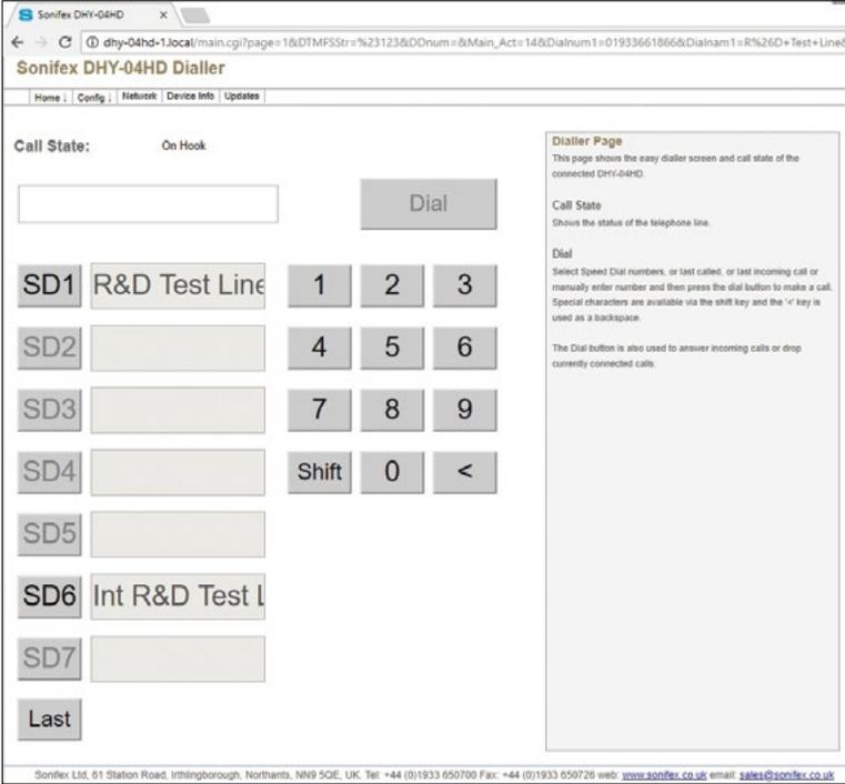
Figure 6-4: Dialler Page – simple screen for making calls – accessed via Home Menu drop-down
