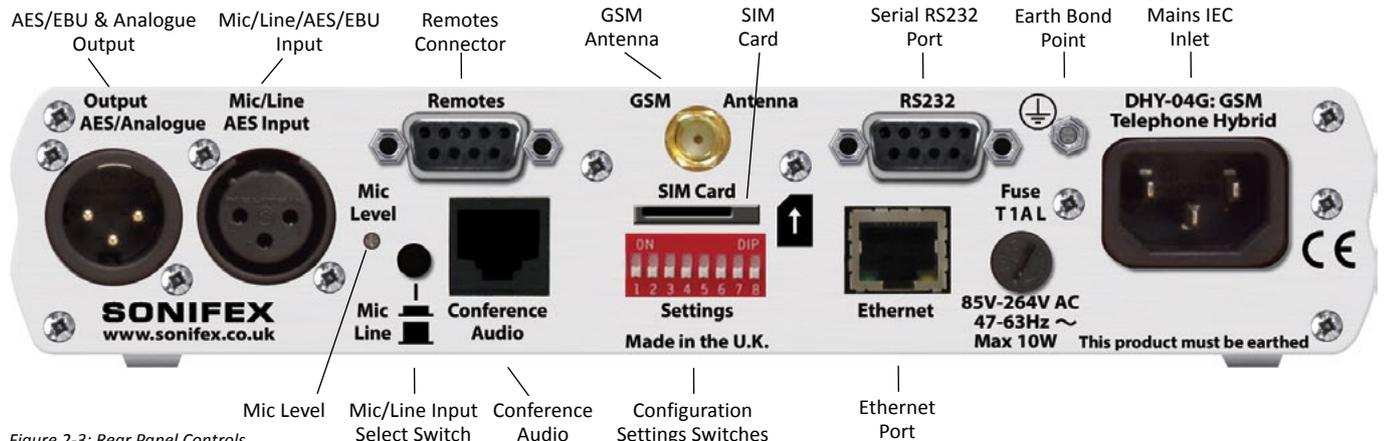
Figure 2-3: Rear Panel Controls
