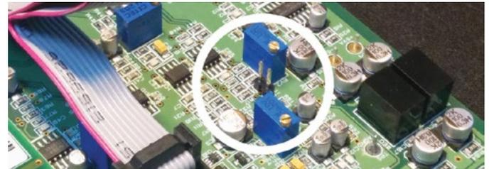
Figure 2-2: Internal Position of Jumper J1
