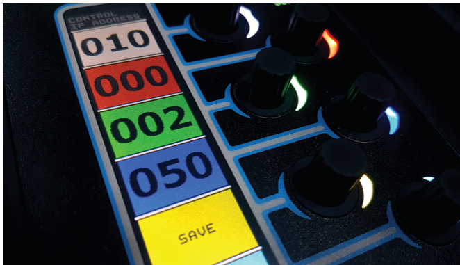
15. Modify the IP address so that it is within the same subnet as your PC, then select 'Save' using the yellow encoder.
