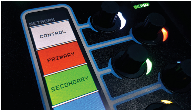
13. This sub-menu shows the available network ports on the commentator unit, select the 'Control' port by pressing the white encoder.
