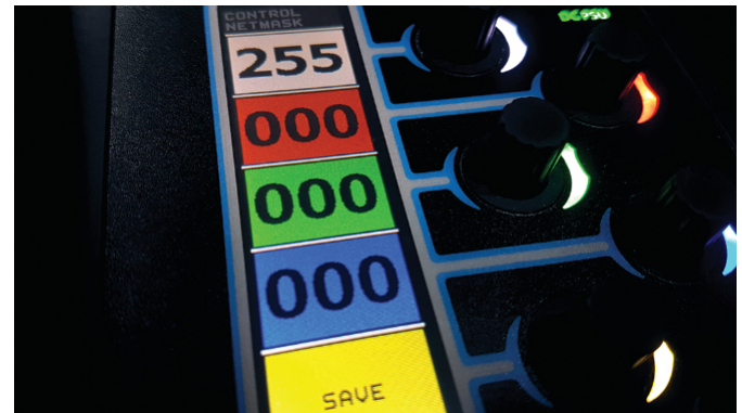
16. This takes you back to the control port sub-menu. Select 'Netmask' using the green encoder, and then change the subnet to match the subnet of your PC, again selecting 'Save' once complete.
