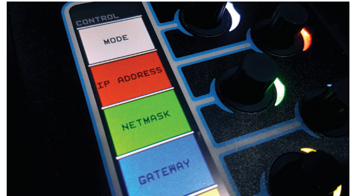
14. This sub-menu shows the IP address settings of the control port, select 'IP Address' by pressing the red encoder.
