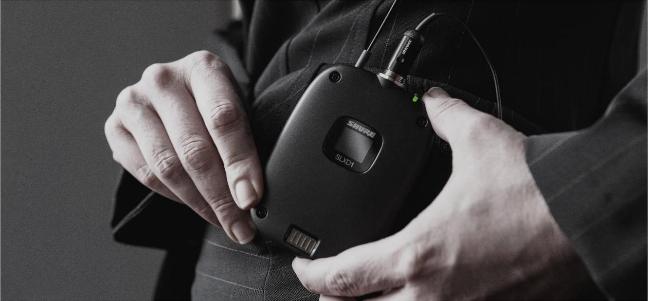
1. Remove the lavalier mic, headset, or earphones and clean separately. Antennas should be left in place.
