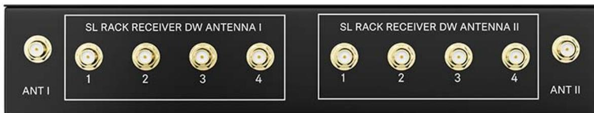
The SL PASC 4 is a passive four-way true diversity antenna splitter/combiner for the SpeechLine Digital Wireless microphone series. It is used to distribute the antenna signals from up to 4 SpeechLine Digital Wireless radio links. In combination with the AWM 2 or AWM 4 remote antennas, the number of required antenna cables is reduced to a minimum. The rack receivers are connected to the SL PASC 4 using the supplied SMA-R cables.
