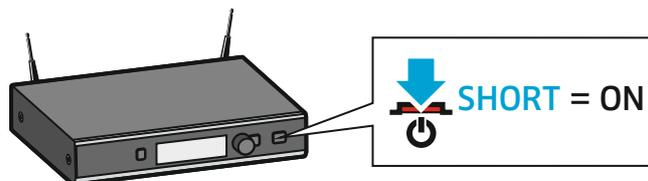
The display panel first shows a logo and then the home screen appears. The status LED indicates the current status of the receiver. The radio link to the last paired transmitter is established automatically as soon as the transmitter is switched on.
