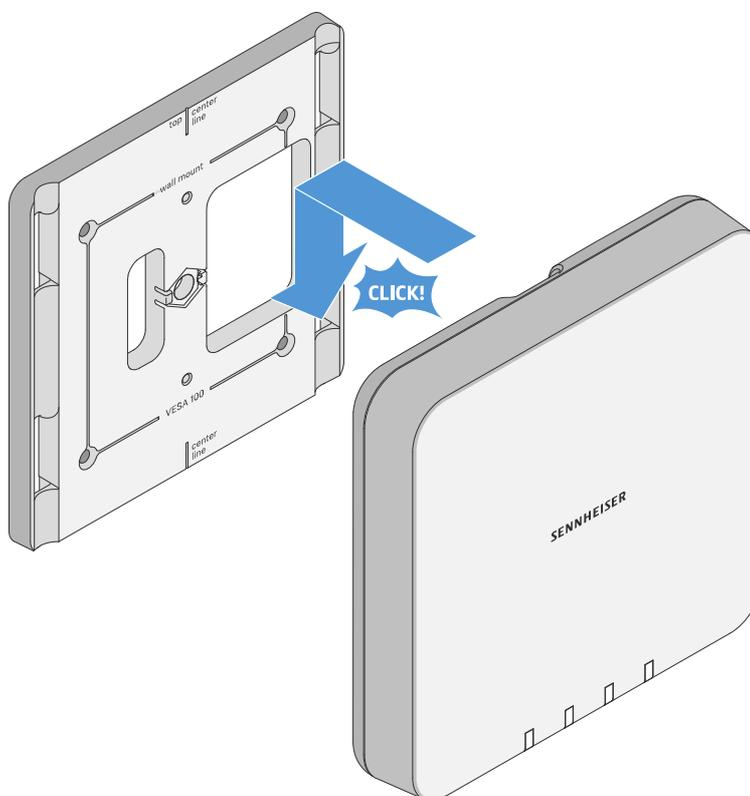
Insert the receiver into the mounting frame as shown until you hear it click into place.
