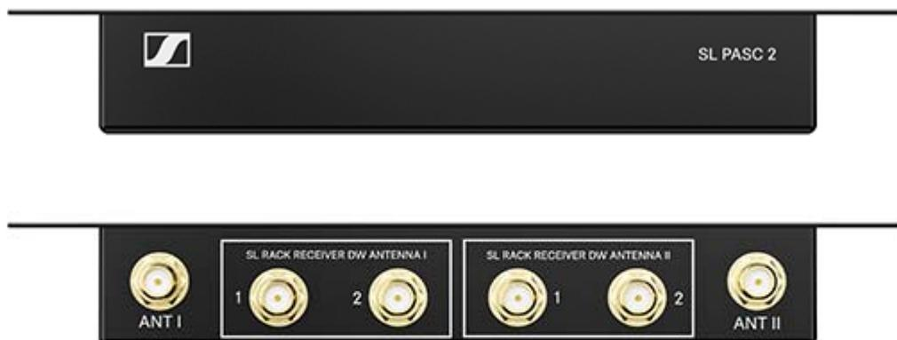
The SL PASC 2 is a passive two-way true diversity antenna splitter/combiner for the SpeechLine Digital Wireless microphone series. It is used to distribute the antenna signals from up to 2 SpeechLine Digital Wireless radio links. In combination with the AWM 2 or AWM 4 remote antennas, the number of required antenna cables is reduced to a minimum. The rack receivers are connected to the SL PASC 2 using the supplied SMA-R cables.
