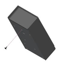
STEP #1 Start the screw into the bottom of the SYSFLEX unit but do not install it all the way.
