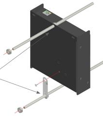
Cut outs and mouting tab may be used to suspend the unit above the ceiling using hanger wire.
