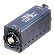
Female XLR chassis connector 110  $\Omega$  input - female BNC 75  $\Omega$  output. For matching balanced 110 ohm digital audio circuits to unbalanced 75 ohm video circuits.
