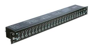
The NYS-SPP-L1 is a economical and remarkable sleek designed 1/4" modular Patch Panel for 19" rack mount (19" x 1U) with a reinforced metal housing. Each of its 48 PCB wired balanced channels (24 front pairs and corresponding 24 rear pairs) can either be grounded separately or in groups determined by the user.
