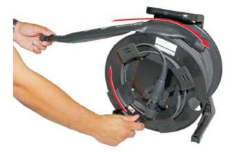
**A** Reel up attached pulling sock flat on to the cable drum being used.
