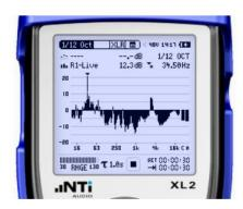
The Spectral Limits Option extends the XL2 function range in both, the sound and vibration mode. It adds noise curves, trace capturing, relative curve display and comprehensive tolerance handling for the FFT Analysis and high resolution spectral analysis up to 1/12th octave. The vibration mode is enabled upon installing the 25-637 Vibration option.
