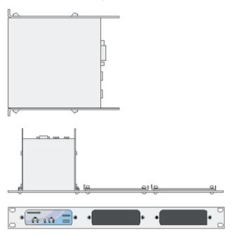
Note that the holes at the rear ends of the brackets may be used as cable tie-off points if desired.
