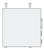
Repeat 2 and 3 for the other side. Push the lid towards the back of the unit as far as it will go, then align the bracket ears with the front edge of the lid. Tighten the screws to secure.
