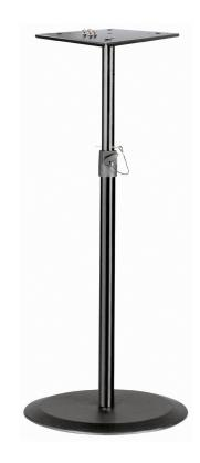
Stable steel stand for monitors with broad completely level round cast-iron base-diameter 450 mm. Rod combination height adjustable using clamping screw and safety splint. For the direct attachment of monitors with 3/8" threaded joint (thread length 12 mm) or to screw in a connector plate 205 x 245 mm for Genelec monitor 1030 or monitors by other manufacturers. Includes 4 thread points and 4 rubber knobs.
