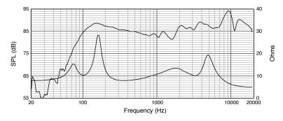
Frequency response in half-space (2pi, mounted in ceiling), impedance at  $8\Omega$  (low-impedance) setting
