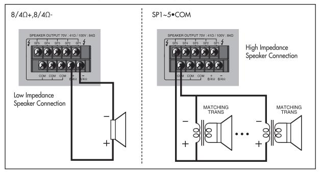
\* Caution: Be careful not to make total impedance of the speaker terminal to be lower than defined impedance in any case. Impedance and output voltage are as the following table:
