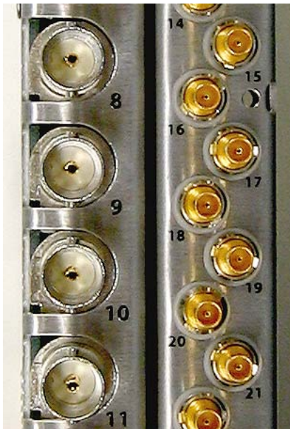
BNC vs. 1.0/2.3 size comparison
