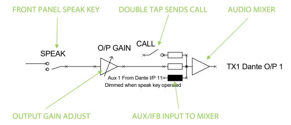
The AUX/ IFB input is a very useful circuit and can be used for example to distribute programme audio to the user connected to the channels output, or maybe a clean feed circuit has been derived from mixing desk or router for onward sending to an outside source and this can be sent to that source via the AUX/ IFB input.
