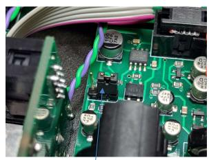
Jumper for Phantom Power ON
