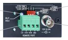
A rear panel three position DIP switch is used to set the sequence mode (+12V ON, +12V OFF, GND ON, Mom/ Maint) which defines how the PS-8RE III will react to the signal presented on its REM input.
