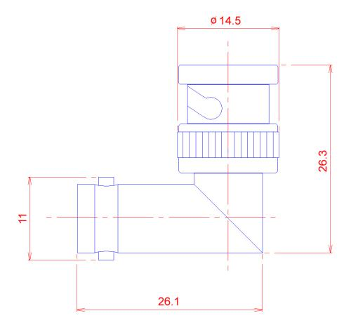
BNC Male to Female right angle adapter for 50 Ohm applications.
