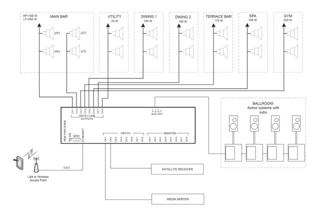
The example above shows an how the eight channels of a CV8125 amplifier may be used to provide audio to different areas of a hotel. All loudspeakers are 70/100 V-line models and the system may be extended to additional speakers in each area as required, provided the total 500 W power capacity of the odd/even channel groups is not exceeded.
