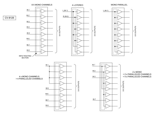
Although the routing options available using the rear panel switches are likely to suit most applications, even greater flexibility of routing is available using the web browser pages, which allow any amplifier channel to be sourced from any physical input (or none) without restriction.
