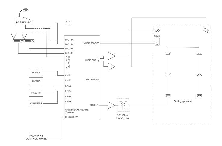
The CX335 is normally connected into the audio system between the mixer, zoner or other sound source selection component, and the main power amplifiers. The connection is entirely straightforward; the active audio source feeds the CX335's inputs, and its outputs feed the power amplifiers' inputs. All interconnections are stereo, and
