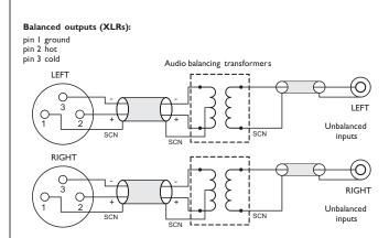
If transformers are not available, a balanced source may feed an unbalanced input directly as long as care is taken over how the connections are made. A variety of design techniques are in use to implement balanced outputs in audio equipment, and some designs require different wiring protocols to others. Installers are advised to check the manuals with each item for guidance on how the outputs should be connected to an unbalanced input.
