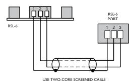
Before the RSL-6 will operate, the **RSL-6** port must be enabled by setting the adjacent **LOC/REM** push-button switch ([16] on page 9) to REM (i.e., pressing it in). In this setting, the front panel **MUSIC LEVEL** and **SOURCE** controls become inoperative.
