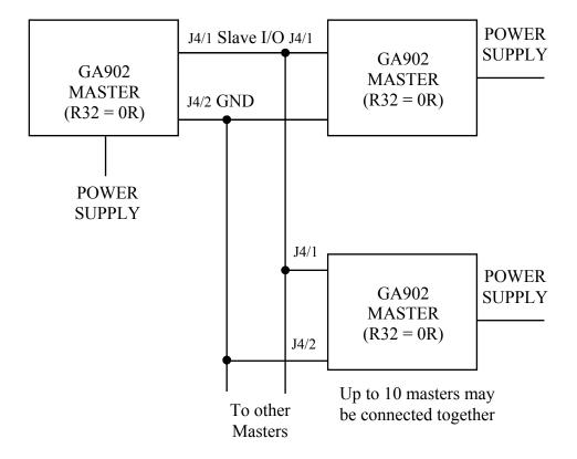
A GA902 master may be converted to a dumb master by removing the OR wire link from position R32 and replacing it with a diode such as a IN4148 or IN4001 etc.
