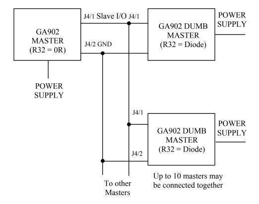
An example is shown below where there is a mixture of masters, dumb masters and slaves all connected together to form a warning system: -
