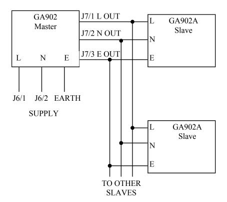
A GA902 (master) may drive up to 10 GA902 master units such that if any master unit is on then all the masters will also switch on.
