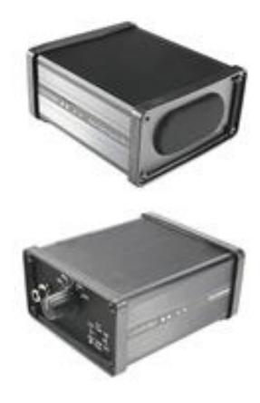
The test system consist of two units, the signal generator and the detector. The Canford Audio phase check system allows fast testing of the polarity of acoustic transducers, microphones and electronic devices. Sophisticated signal processing allows fast and accurate determination of the absolute polarity, unimpaired by passive crossovers or signal waveform distortions produced by the device under test.
