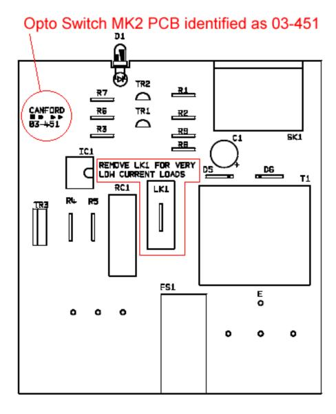
The switcher can supply a current of up to 8mA when switched off, so it may not be suitable for driving very light loads e.g. some LED lights etc.
