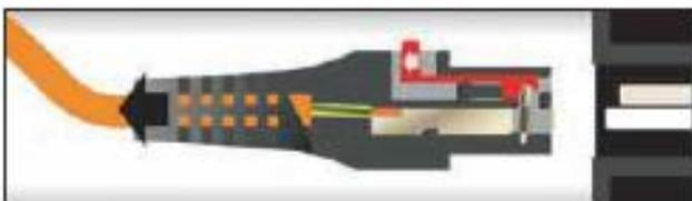
Sliding back the 'red' tab releases lock mechanism allowing disconnection from the inlet.
