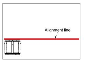
ii. Using the large spacer, place the second wall mount as shown whilst being careful to keep on the alignment line.
