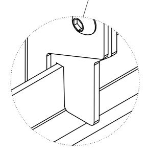
**Note:** Ensure the bottom interface arm hooks are properly mounted onto the wall plate.
