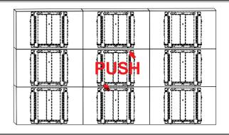
**Note:** Push at the top and bottom of the screen on the bezel. To avoid any screen flexing (and when spacers have been used) apply light pressure in-line with the interface arms, pushing alternative arms at the top and bottom simultaneously (see fig. 1).
