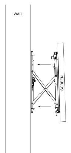
**Note:** Safety screws need to be in the unlocked position. Tighten safety screws once <u>all</u> flat screens are mounted and aligned with each other.
