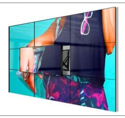
iii. When servicing is complete, push the screen back and click into place.
