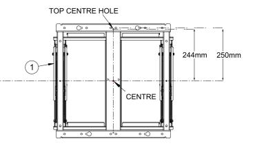
iii. Fix the wall mount to the wall (use the horizontal line as a guide), using the fixing holes with suitable wall fixings (not supplied).
