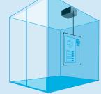
Installation behind a metal panel or metal trim will rarely produce an effective magnetic field with any amplification method. Please contact Ampetronic for detailed guidance on the best installation method for your lift car or industrial environment.
