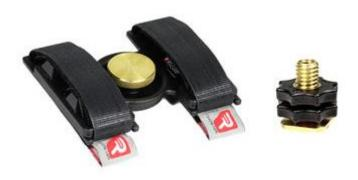
The Rycote Wireless Receiver Camera Bracket MKII is a universal wireless microphone receiver holder used to mount receivers onto a 1/4" mount or flash shoe on any camera. The bracket features a brass thumbwheel which makes secure mounting easier as well as larger overall dimensions to improve compatibility with receivers. As with the Mk I it has 4 soft grip pads and hook-&-loop straps for securing receivers in place. A shoe mount is included.
