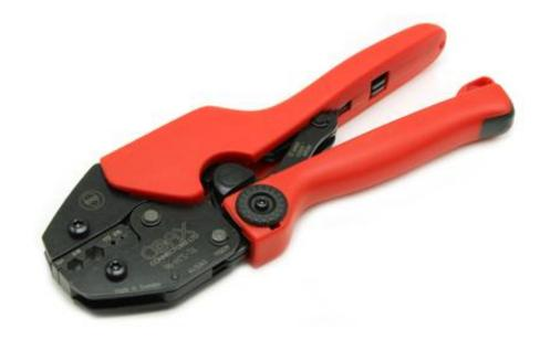
Ratchet Crimp Tool complete with die set for terminating COAX 75 ohm BNC, Micro BNC and DIN 1.0/2.3 connectors to Canford group Q broadcast cables as well as Belden 1505F. Die set has the following cavities:
